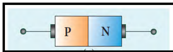
Fig 10: p-n junction diode (a) Schematic representation
